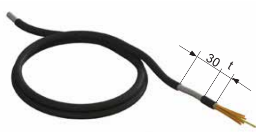
Figure 25: Strip 30 mm from the EMC cable before connecting to the cable terminal board. Dimension "t" corresponds to the approximate gap from the fastening clip to the cable terminal
